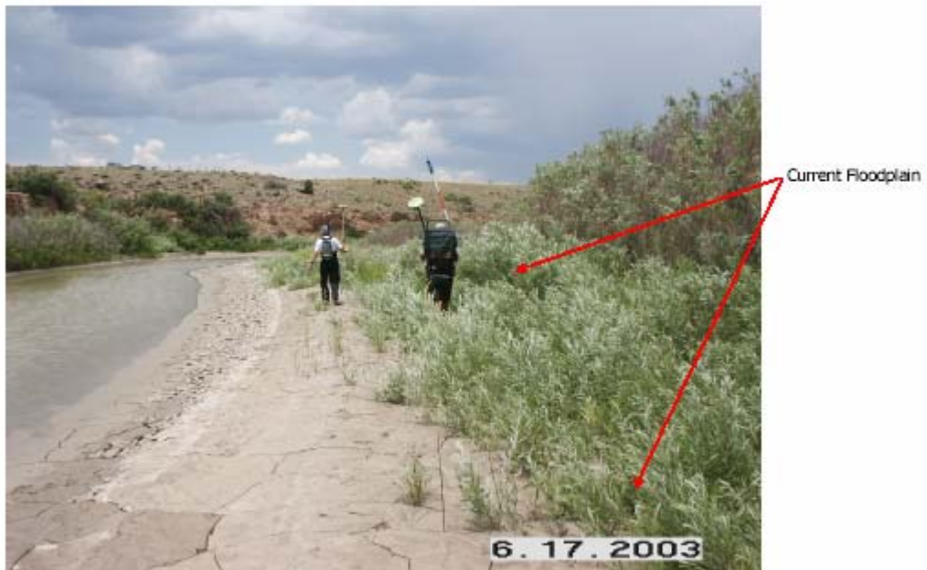
Figure 17 – Surveying the floodplain downstream of cross section 17. Note vegetation establishment. View is looking downstream on right bank of river. (June 17, 2003 – Discharge at Bedrock gage = 40 cfs).
